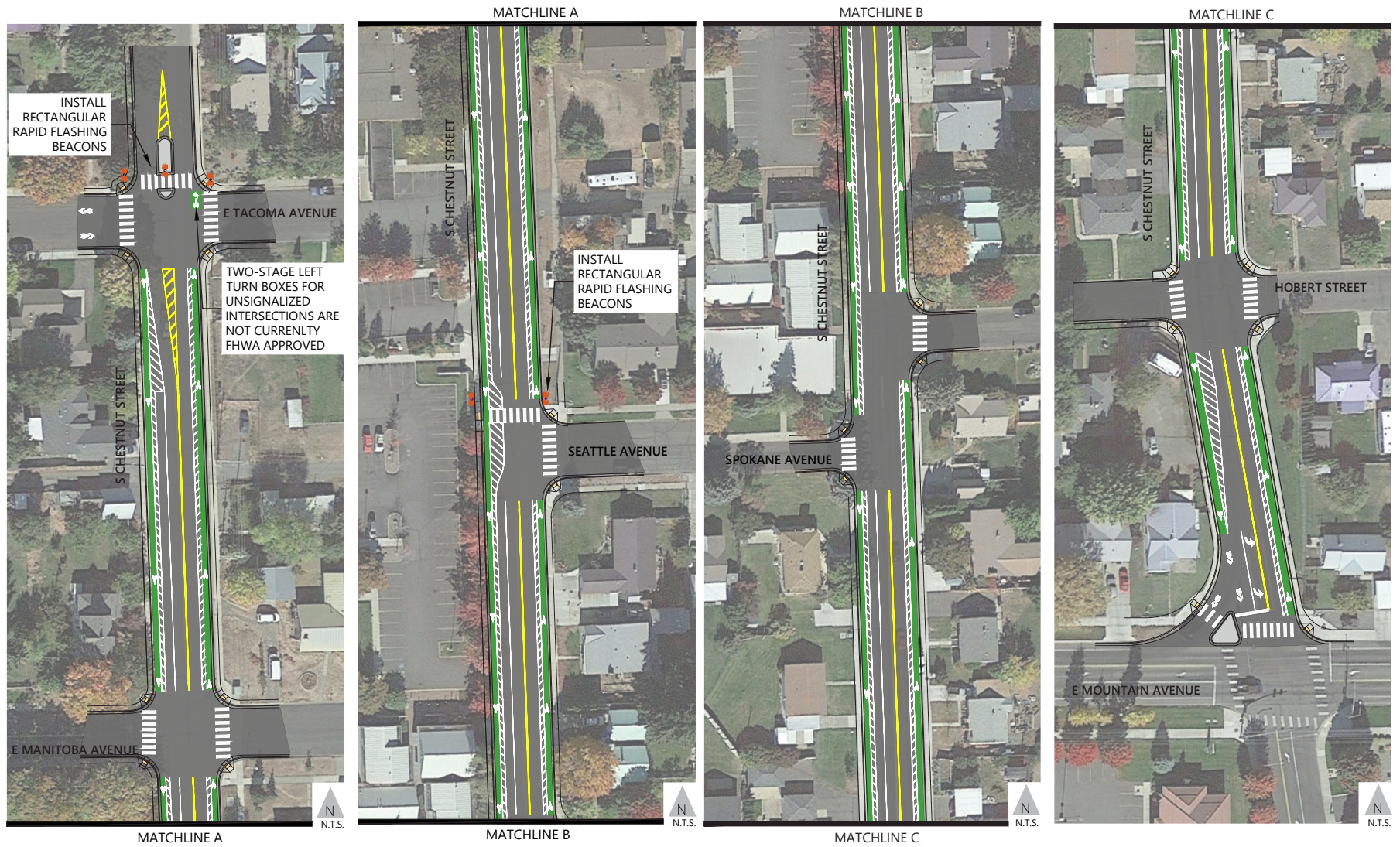
Figure 11 - Conceptual Design of Buffered Bike Lanes Along S Chestnut Street, Including RRFs and Crossing Islands
