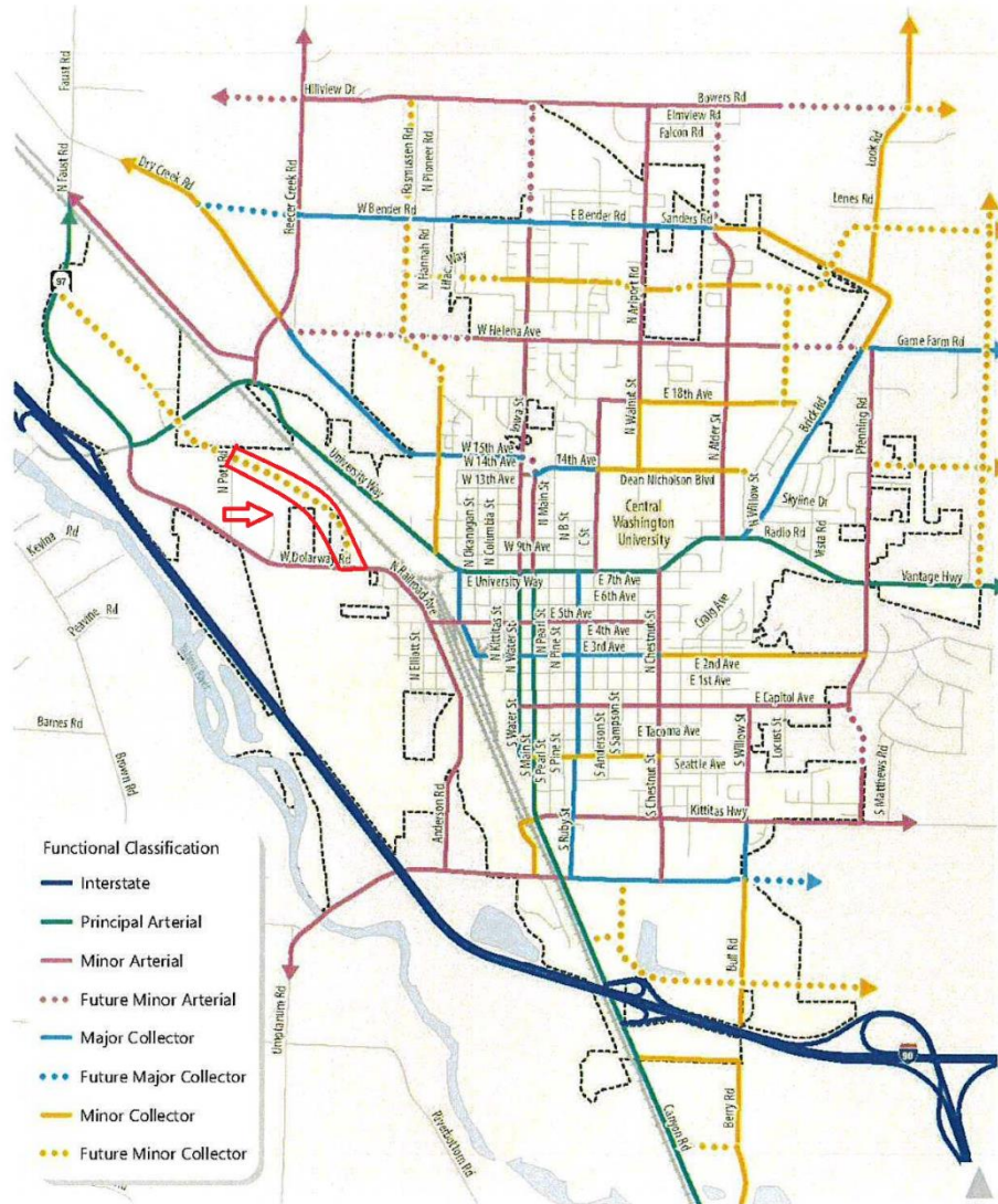
Figure 13. Roadway Functional Classifications
