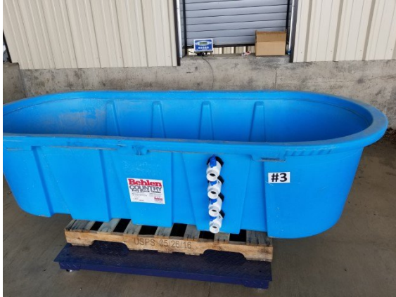
Step 7, get tare weight on all tanks
