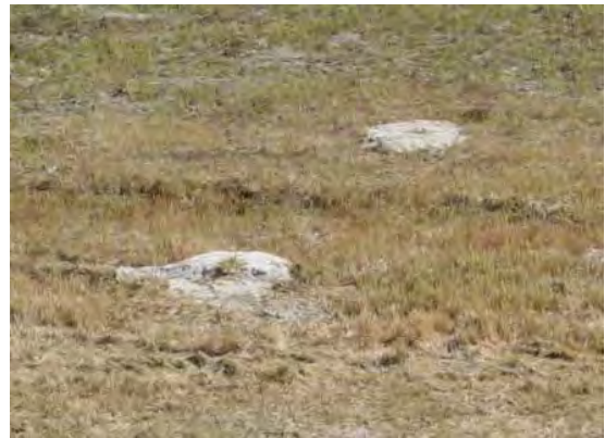
Figure 2.41 Evidence of sandboils. (IN)
