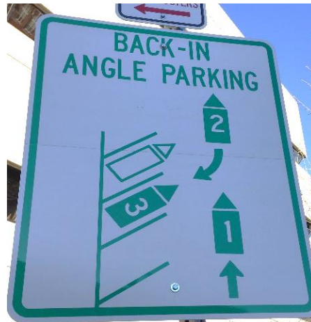
Many cities utilize back-in angled parking as a means to improve safety and convenience. Clear sightlines and eye contact between all road users ensures safer parking maneuvers. Clear signage is instrumental in overcoming user confusion. Salt Lake City (left) and City of Spokane (right).
