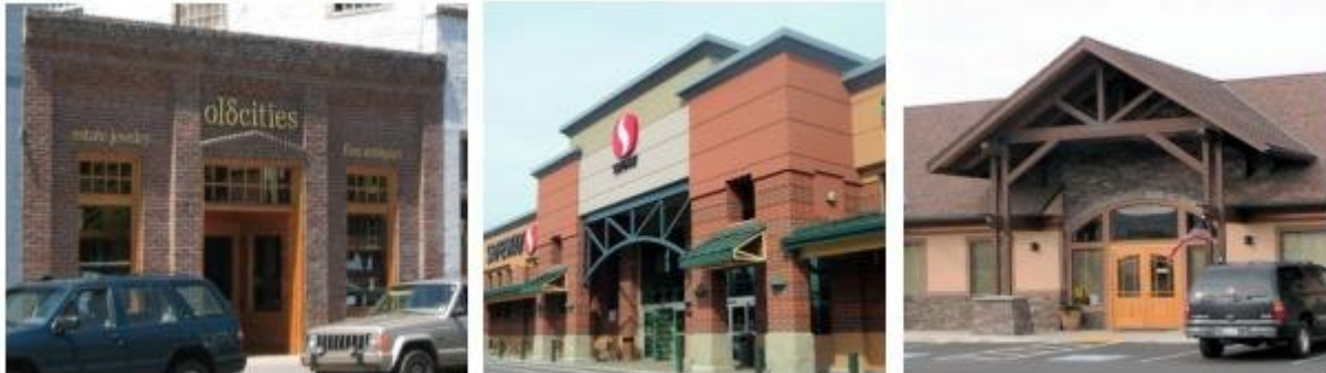
Figure 15.530.040(C). Facade details examples. The building on the left uses decorative windows and doors, decorative roofline and columns, and decorative materials (brick and wood). The center image uses a decorative entry feature (metal feature over entry), decorative weather protection and lighting, and decorative use of brickwork. The right image uses decorative wood beams over the entry, decorative windows and doors, and stonework.
