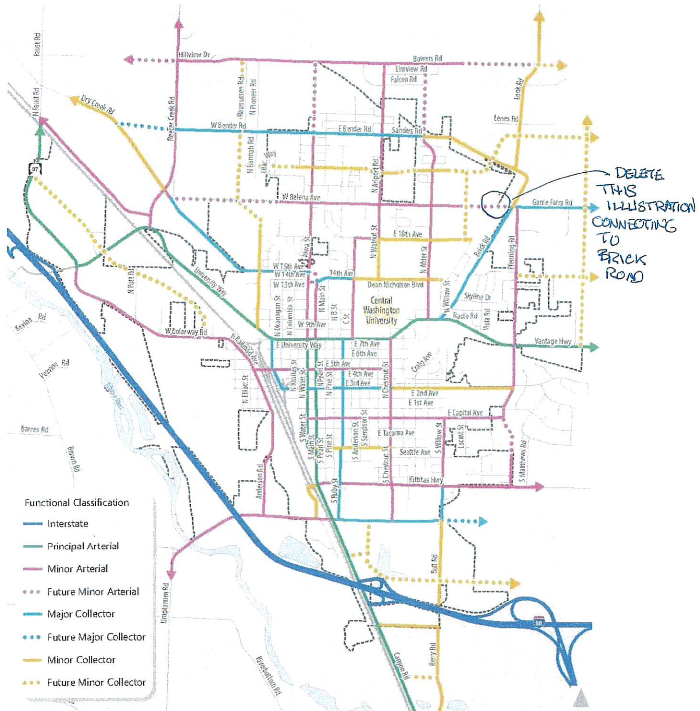
Figure 13. Roadway Functional Classifications
