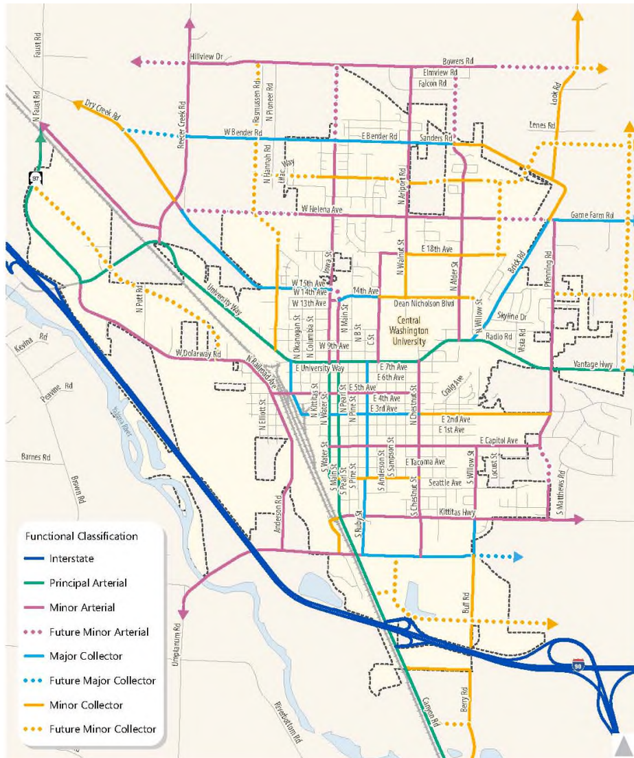
Figure 443. Roadway Functional Classifications
