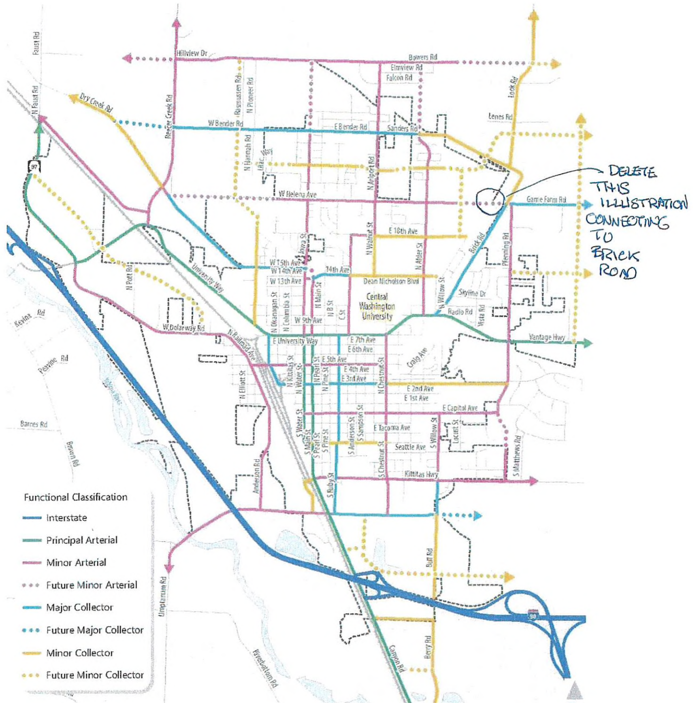
Figure 13. Roadway Functional Classifications
