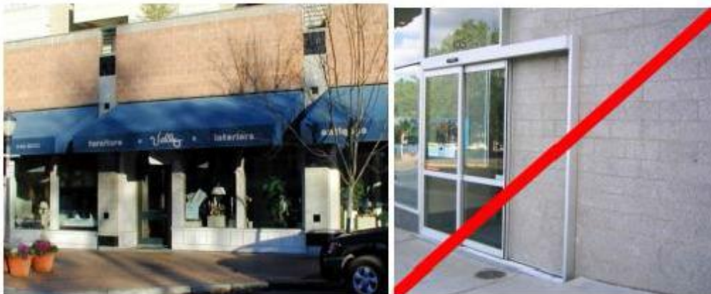
Figure 15.530.050(D). Acceptable and unacceptable concrete block examples. The left example uses a mixture of split-faced colored concrete block and smooth-faced concrete block, together comprising just under 50 percent of the whole facade. The large expanse of smooth-faced concrete block on the right is not desirable for Ellensburg facades.
