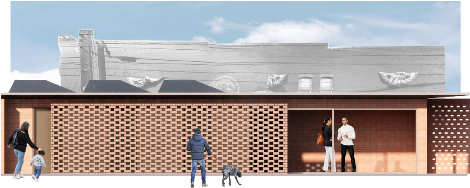
East Elevation (with perforated screen wall)
